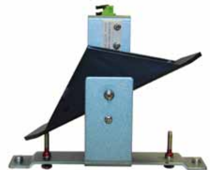
RG1 tipping bucket mechanism
